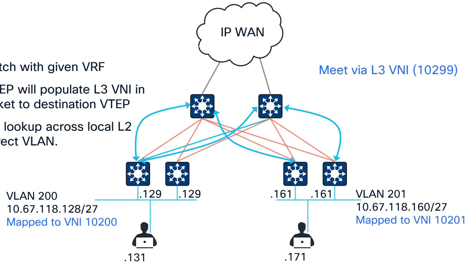
Think of L3 VNI as an inner MPLS label in VPv4 MPLS VPNs; It is used to identify correct IP VRF at the destination switch.
