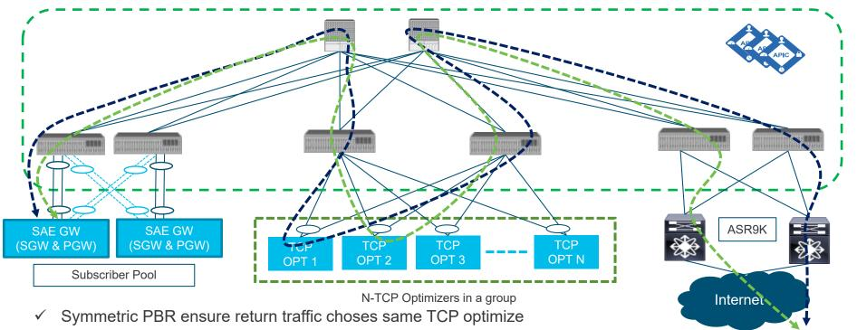
Automatic load-balancing of traffic across different TCP optimizers based on forwarding table hash (Source IP, Destination IP, Source Port, Destination Port)
