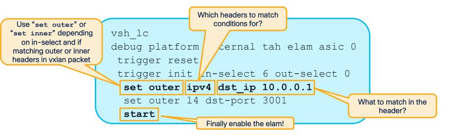
When running stat if Triggered is seen, this means a matching packet was received
