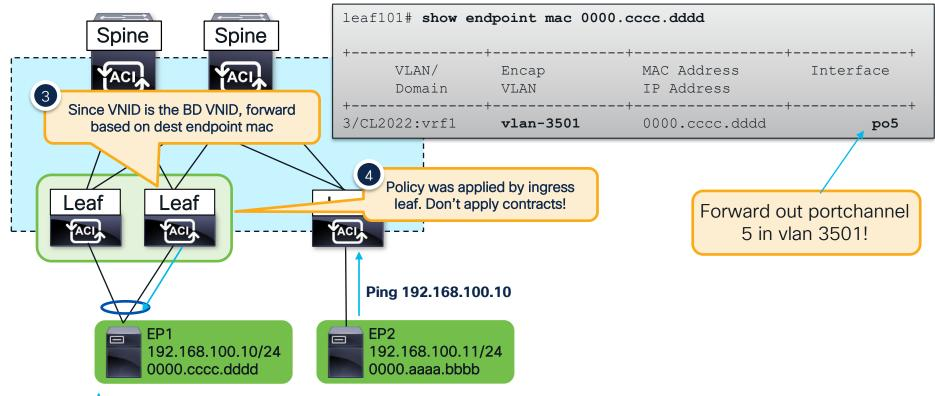
Bridge Domain Settings: Unicast Routing Disable Unknown Unicast Flood
