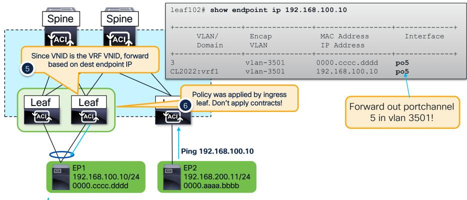
Bridge Domain Settings: Unicast Routing Enabled
