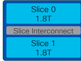
LS3600FX2 – 36 x 100G 3.6T chip – 2 slices of 18 x 100G with MACSEC 9300-FX2 TORs
