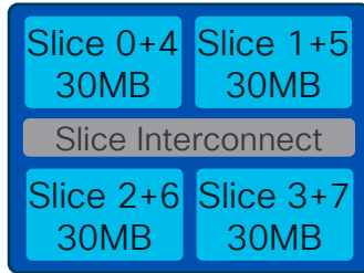
LS25600GX2A 30MB/slice pair (120MB total)
