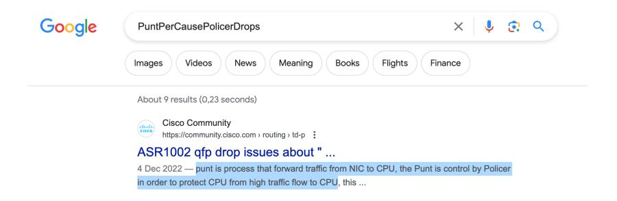
So, there is a rate limiter for punted (sent to CPU control plane) packets which is exceeded
