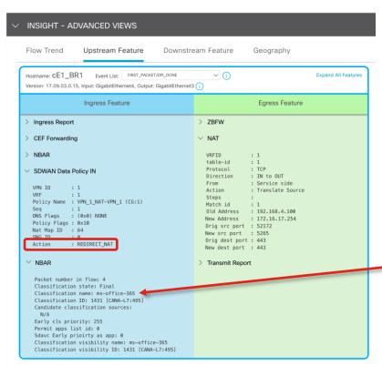
Here you can see DPI misclassified internal application as "ms-office-365" and traffic was sent to DIA circuit instead of overlay tunnel, hence, causing blackholing
