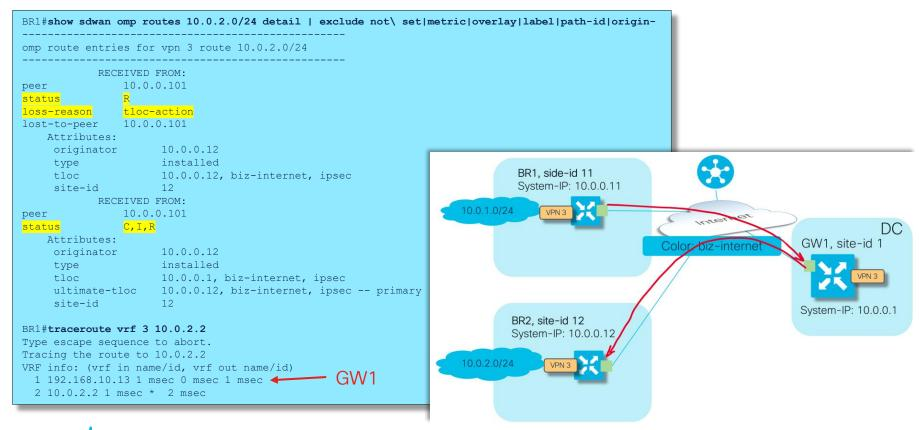
Case 4 ½. Traffic engineering with "set tloc-action". Disjoined underlay. Same control policy, but BR2 connected to a different transport.
