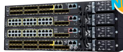
Stackable rack-mount all fiber or all copper Catalyst IE9300
