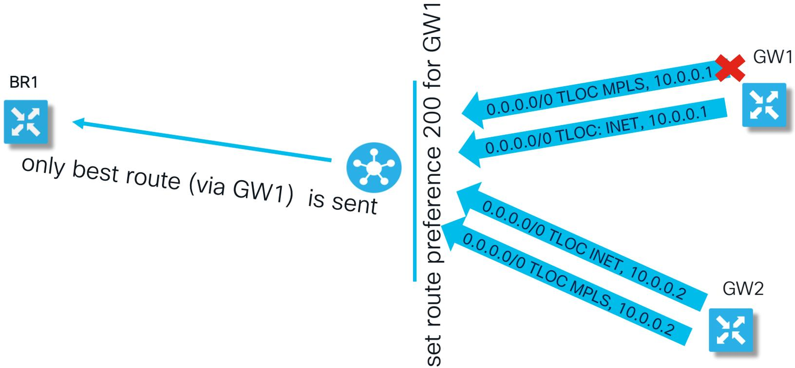
And BR1 can't resolve path via internet because it is connected to mpls color only
