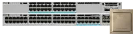
Catalyst 3850 mGig - 2015 UADP 1.1 - 3.0B transistors
