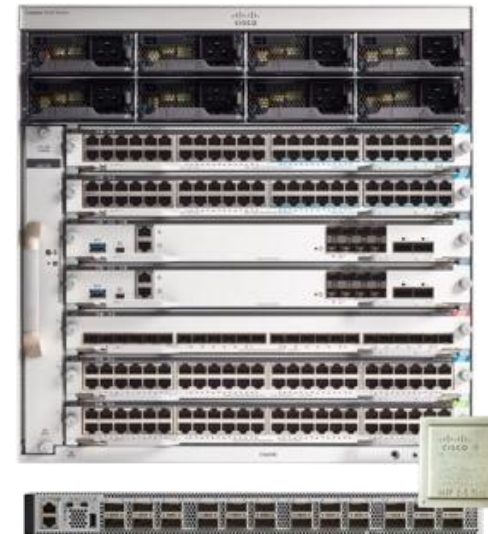
Catalyst 9400/9500 - 2018 UADP 2.0 - 7.5B transistors
