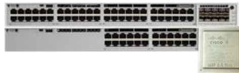
Catalyst 9300 - 2017 UADP 2.0 - 7.5B transistors
