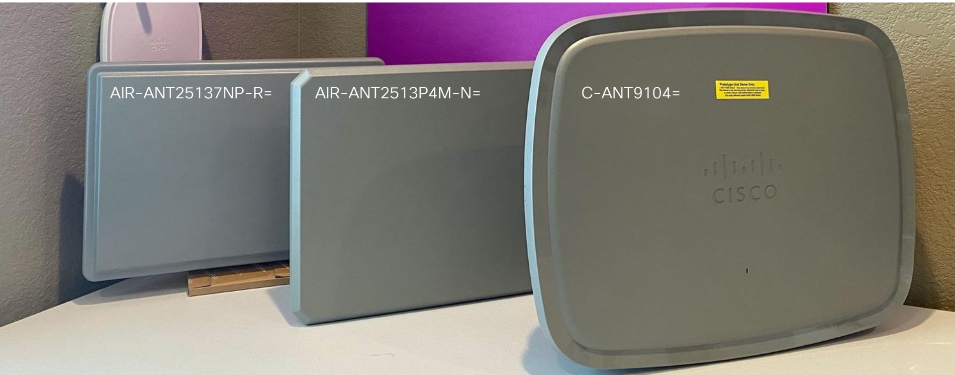
Three generations of High-Density WiFi Stadium Antennas
