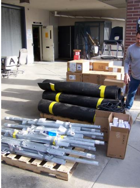
10x Tylon small ballast NPRMs (36"x36") shown knocked down on left along side rubber mats. One 36x36 NPRM assembled with 20cm concrete blocks on right.
