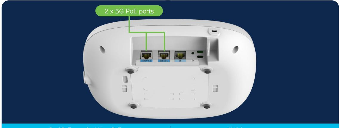
Dual PoE ports for hitless PoE: No reboot required if a port loses power Uplink ports support: 802.3 link aggregation for increased throughput resiliency
