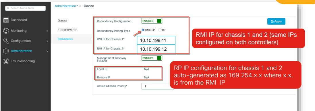
**Note**: RMI can be in the **same VLAN as the wireless management (recommended)** or in a different VLAN. The netmask for RMI is picked up from the netmask configured on the VLAN.
