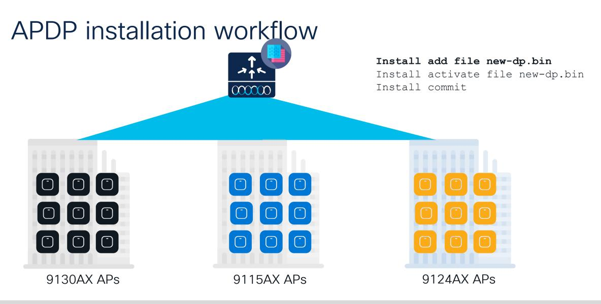
Note: Fixes for the AP installed via APDP will be via AP Service packs like a baseline supported AP.
