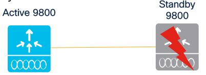
• If the active controller crashes, the standby becomes active. The new active shall assume the role of active and try to detect a dual active.
