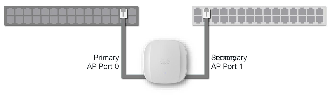
Note: Ensure both switches provide the same power level and have connectivity to the WLC.
