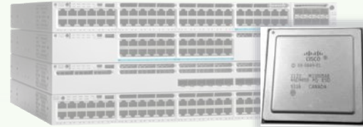
Catalyst 3850 Circa 2013 UADP 1.0 – 1.3B transistors UADP 1.1 – 3.0B transistors 1,490,000 lines of code
