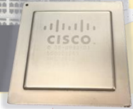
UADP 2.0: 7.46B transistors! UADP 3.0 – 19.2B transistors! 2,160,000 lines of code
