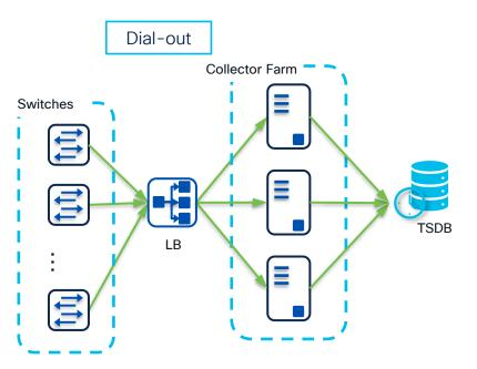
Collectors can be set up behind load balancer, all switches stream to the same VIP of collector
