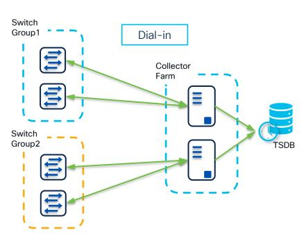
To distribute the workload, the collectors need to dial into different switch groups, extra effort to keep the sensor configure synchronized across the cluster
