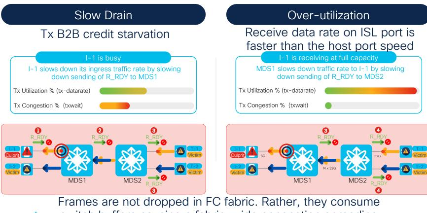
switch buffers causing a fabric-wide congestion spreading
