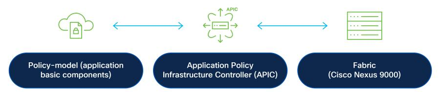
The unified point of automation and management for the Cisco ACI fabric, policy enforcement and health monitoring for physical, virtual and cloud infrastructures
