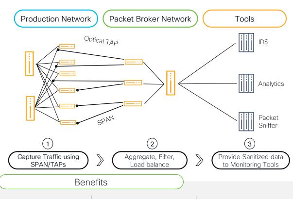
Nexus switch functions as packet broker
