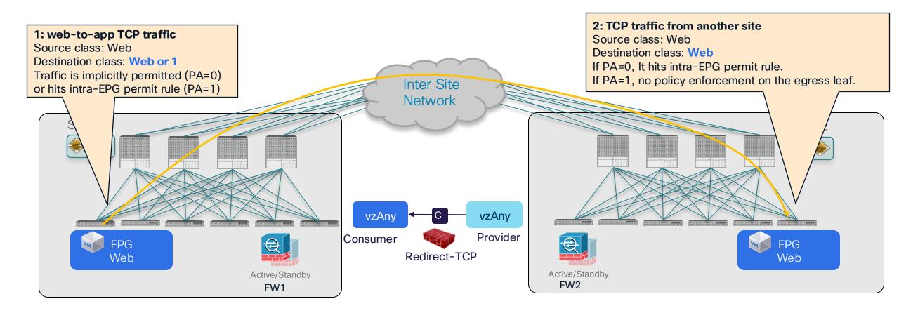
Bypass firewall for specific EPG-to-EPG traffic
