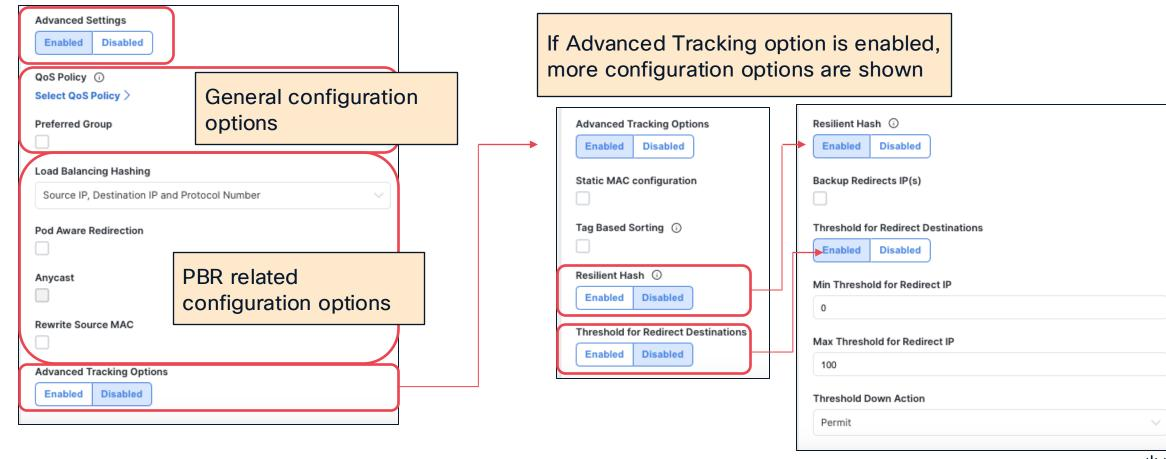
2: Configure a Service Device template for site level (1/3)
