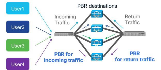
Some traffic could be load-balanced to different PBR nodes that don't have existing connection info.
