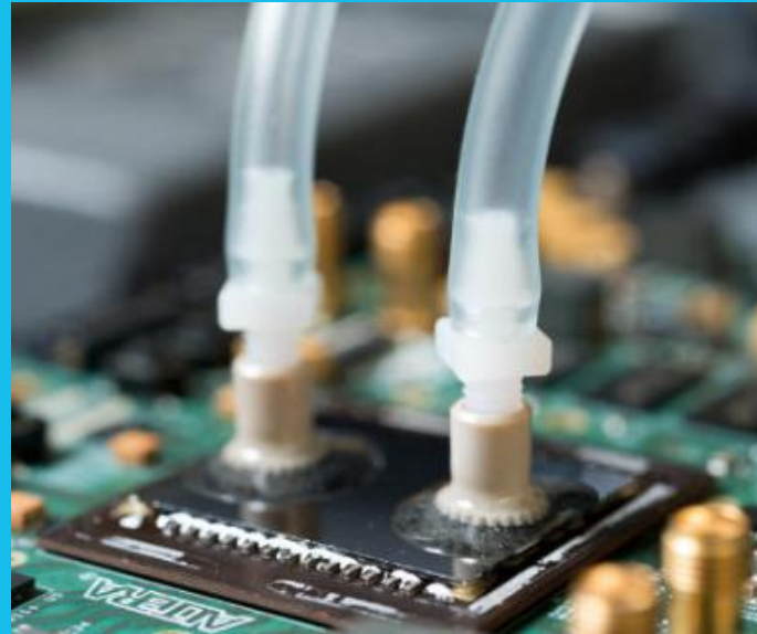
Direct to Chip 150 kW per rack
