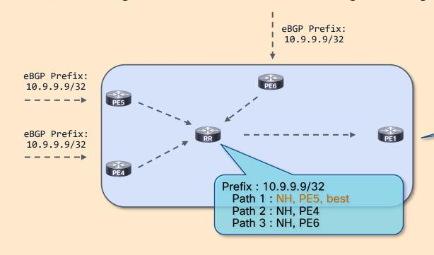
But PE6 is closer (IGP-wise) than PE5 as exit router
