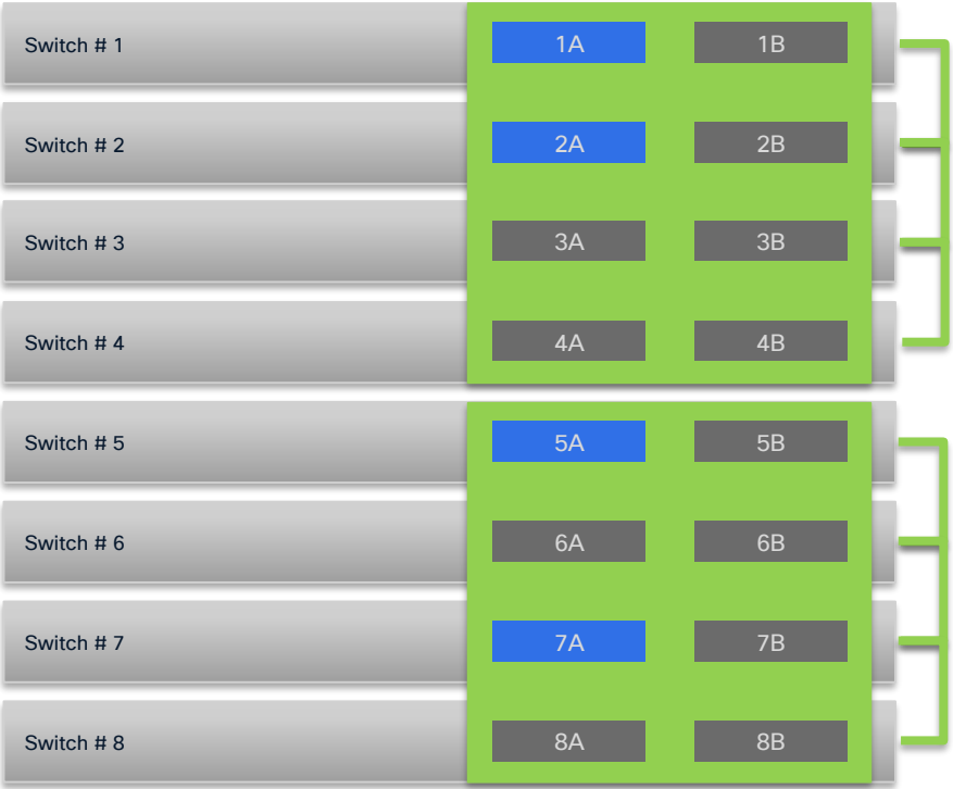
8 x C9300X switch stack 2 StackPower Domains 4 Active PSUs
