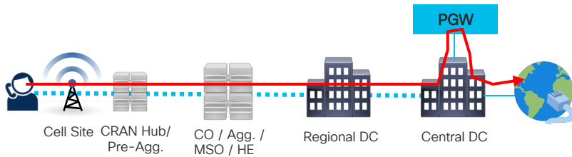
Centralized, Appliance Based Mobile Gateway
